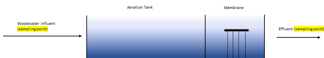
Figure 4.48. Schematic diagram of the MBR system tested in the study.
